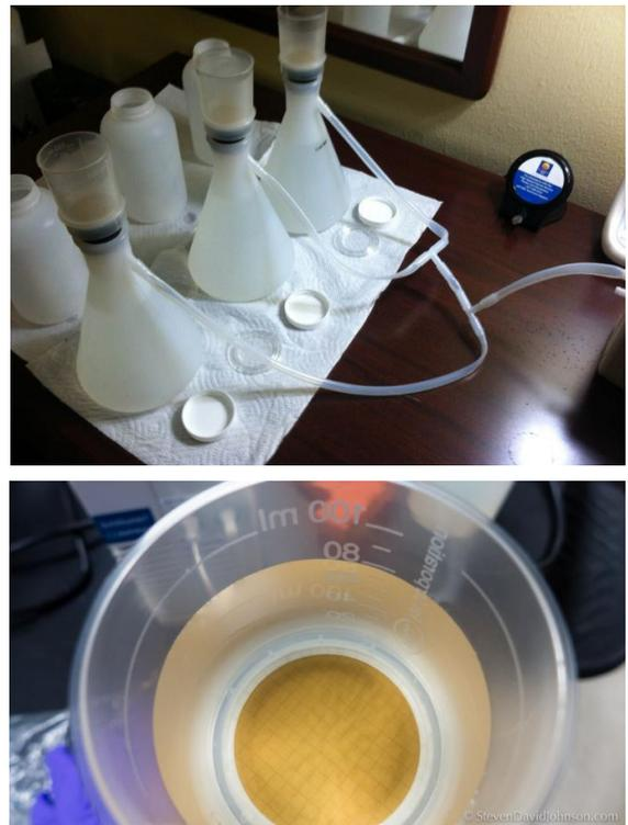
Fig. 1. Filtration system for eDNA capture. *Top*: Stream water is collected in 1-L bottles and poured into filter cups attached to a vacuum flask. *Bottom*: The ultra-fine filter paper captures DNA, sediment, and other microscopic debris in the water.
